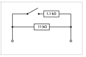
The resistor circuitry is designed such that the NAMUR specifications can be satisfied. An operating voltage of 8.2 VDC must be provided for NAMUR-compliant operation. A resistance of 11 k $\Omega$  is present in the circuit when the switch contact is open. The resistance is 1 k $\Omega$  when the switch contact is closed. Other resistance values can also be realised.
