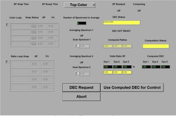
Automated dye efficiency compensator display
