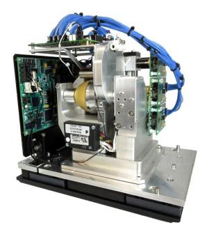
The compact sensor design uses Honeywell's EDAQ based MXIR architecture, which allows the sensor to be mounted in-board on the Experion MX Q4000 O-Frame scanner.
