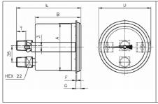
PDR02...H: for panel mounting, with front ring and hangers, connection at back
