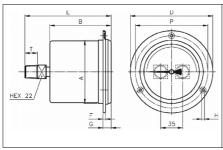
PDR02...N: for panel mounting, with three-hole front ring, connection at back
