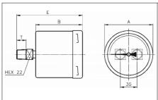
PDR02...M: for pipe mounting, connection at back
