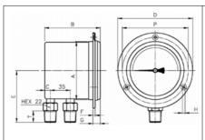
PDR02...O: for pane I mounting, with three-hole front ring, connection at bottom
