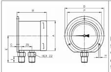
PDR02...L: for wall mounting, with rear rim, connection at bottom
