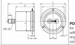
PDP02...N for panel mounting, with three-hole front ring, connection at back
