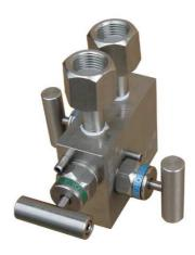
The 3VD-35 valve block is used to shut off the connection to the process and to equalize the pressure between the two inputs of the differential pressure gauge before the actual measurement.
