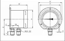
PDP02...L for wall mounding, with rear rim, connection at bottom
