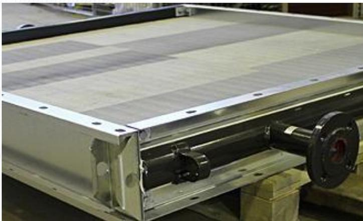
**Original Steam Coils** for pulp dryer heat exchanging units.
