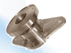
Rotary joint, provides a mechanical seal between a stationary supply pipe and a rotating drum or cylinder to permit the flow of heat transfer media, or just water into and/or out of the rotating element.
