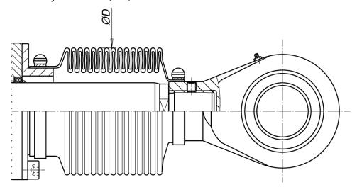
Fastening of the protective bellows, case 2. To the cylinders: 100/65, 125, 160, 200 and 250.
