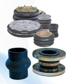
Bellows for expansion joints and in compensators are muffling machine and process vibrations. They can be used to compensate, mounting inaccuracy, to connect moving machine parts to static pipe lines or as sealing elements where pipe systems pass through walls.
