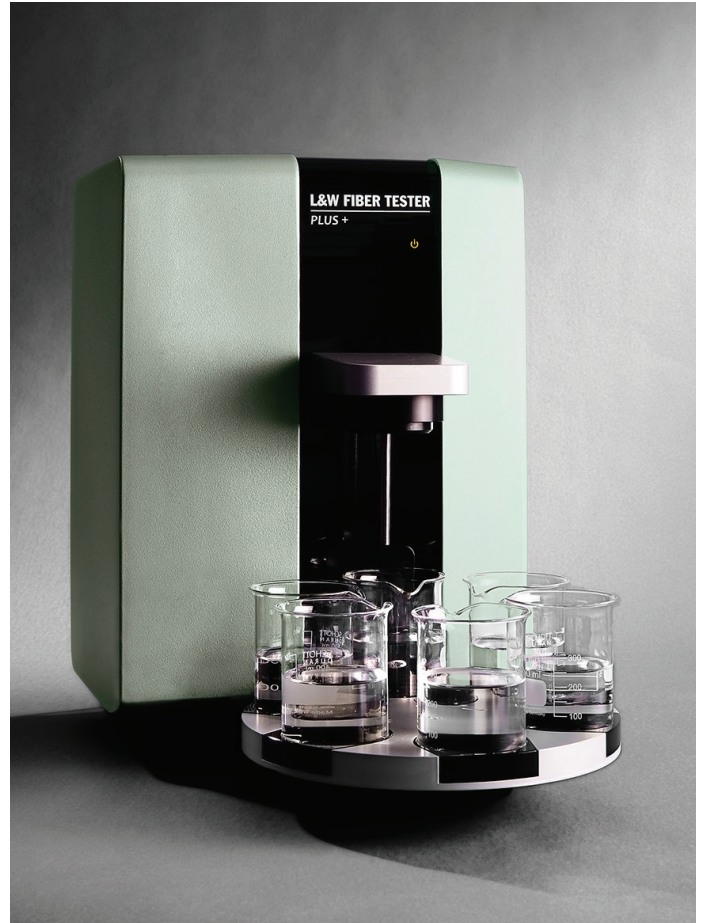
L&W Fiber Tester Plus is a bench-top model, and is easy placed in any laboratory.
