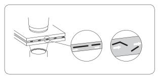
3. For measurement accuracy, a very small distance between the plates is needed. The fibres are then oriented in two dimensions, which enables L&W Fiber Tester to make a correct measurement.
