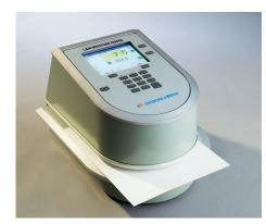
After the weight is registered, the operator puts the sample into the measuring gap.
