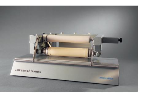
With L&W Sample Trimmer, you can cut a 300 mm wide sample strip from most paper or board samples. This sample can then be tested in L&W Autoline or L&W TSO Tester.
