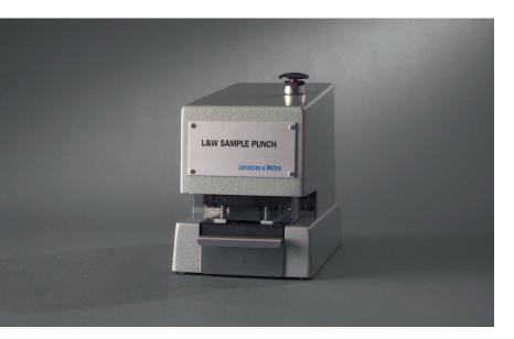
L&W Sample Punch is used for easy and rapid preparation of accurate test pieces for use in tearing tests, bending resistance tests, folding strength tests, or L&W Autoline Elrepho Module. It is pneumatically operated and the specially designed sample holder ensures extremely good cutting results on both thin and tough paper.
