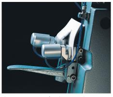
The average amount of work consumed to tear the sheets divided by the total tearing length, is the internal tearing resistance.
