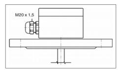
Process connection: flange acc. to DIN EN 1092 DN50...DN200, PN6...PN40 flange acc. to ANSI 1 1/2"...8", #150 RF, #300 RF Material: stainless steel 1.4571 Temperature range: **Connection codes:** FD = DIN-EN flange FA = ANSI flange
