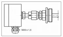
Process connection: Tank fitting G 1 1/2 or G 2 stainless steel 1.4571 or 1.4404 Material: Temperature range: -30...+150°C **Connection codes:** G 1 1/2: TG40 G 2: **TG50**
