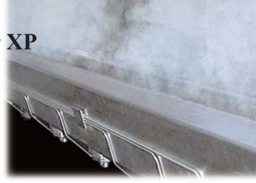
The Calendizer XP optimizes the finishing process with moisture gradient calendering to produce a uniform sheet to improved printability.
