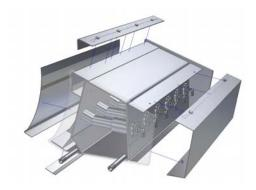
The patented screen plates are custom designed to distribute steam evenly at the optimum, application-matched velocity. They are engineered to prevent fibers from entering the Devronizer, and are removable in Couch, Press and Yankee applications. Adjustable edge deckles are included, when required to facilitate frequent heating width changes.
