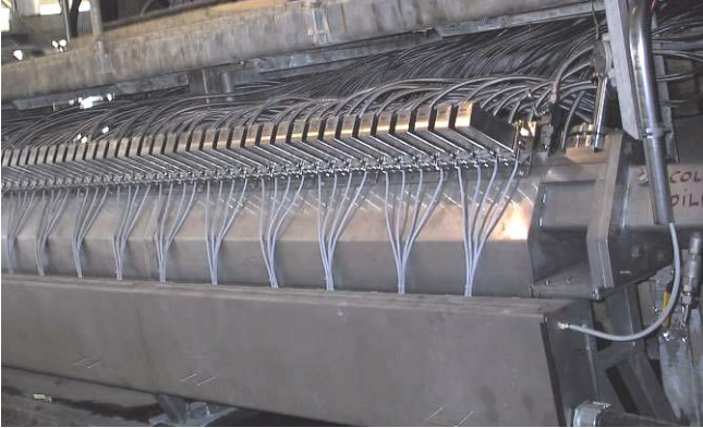
Model 9177-20 installed on a Mitsubishi Heavy Industries MJ Flo dilution header shown with optional cable support tray
