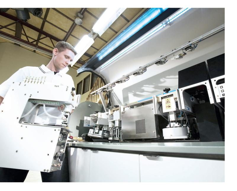
L&W Autoline is an automatic paper testing laboratory providing reliable, accurate and precise information about the quality and condition of the paper. A proven solution at more nearly 500 worldwide locations, L&W Autoline can perform almost all quality testing, prepare reports, archive data, and communicate with other devices that monitor process parameters with little operator involvement.
