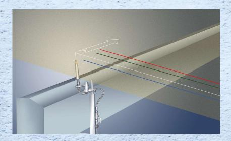
Successful tail feeding is based on accurately controlled tail cutting. Fastpap WetCut is a wetend tail cutter which represents the greatest expertise in its field. With a press of a button it moves to a pre-programmed tail width and, after threading, it quickly widens the web.
