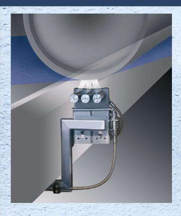
Difficult conditions in the forming section require a fabric cleaner to be consistently reliable. Fastpap FormerSprint is a dependable cleaning system, which improves machine runnability and prolongs fabric lifetime by maintaining its air permeability. A perfectly clean fabric enables faster running speed and minimizes web breaks.
